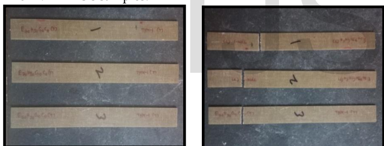
Fig.4.1: Tensile test specimen before and after test.
